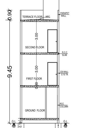
SECTION AT A-A FOUNDATION TO STRUCTURAL DETAIL
